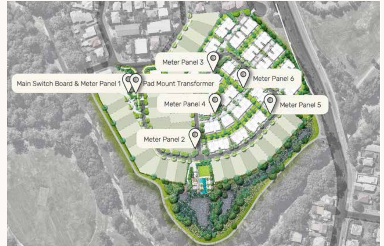
Figure 4: Location of the Meter Panels
