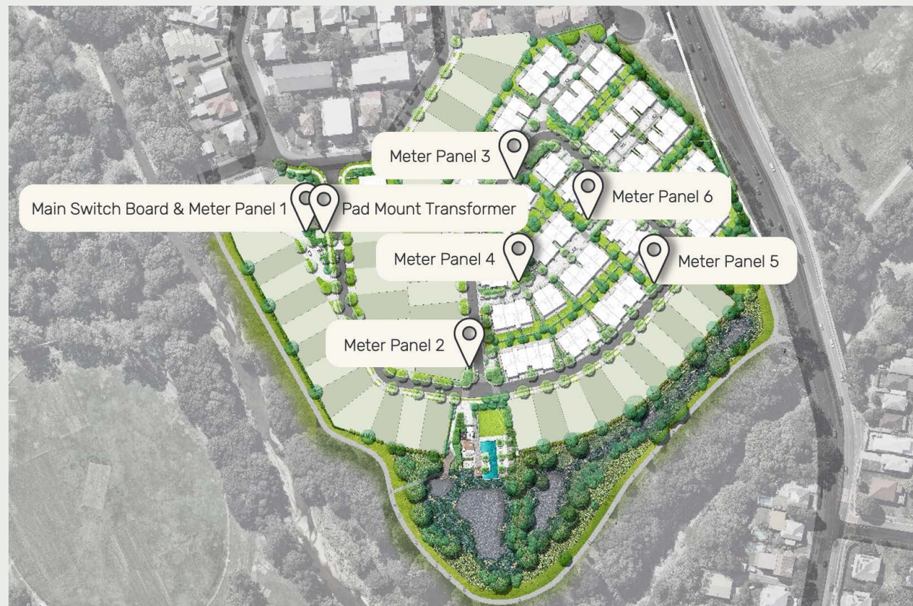
Figure 3: Location of the Meter Panels
